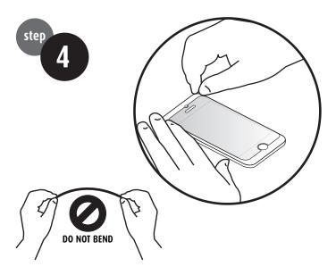
If you are not happy with the alignment, adjust the position by very gently & carefully peeling back the Gecko tempered glass guard from any corner. Repeat step 2 until you are happy with the alignment. IMPORTANT: Do not bend the guard as it may cause it to shatter.
