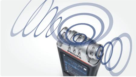
Several key components are needed to record music as naturally as possible in studio-like audio quality: high signal-to-noise ratio, highly dynamic microphones to capture soft tones as well as loud drums, a high-quality microphone suspension to avoid pickup of grip noise, a strong left and right channel separation for human ear live-like effect.
